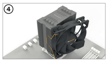
Fasten the 120mm fan onto the cooler unit using fan clips. Connect the fan to the motherboard's PWM signal.
