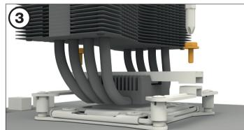
Position the cooler mounting bridge centrally on the cooler. Next place the cooler unit onto the CPU. Insert the mounting bridge fastening screws from above into the cooler mounting bridge and then screw these alternately tight. You can use any cross-tip screw-driver for this.
