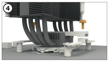
Position the cooler mounting bridge centrally on the cooler. Next place the cooler unit onto the CPU. Insert the mounting bridge fastening screws from above into the cooler mounting bridge and then screw these alternately tight. You can any cross-tip screwdriver for this.
