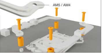
Place the four AMD spacer nuts onto the backplate bolts protruding through the front side and affix both long AMD mounting brackets with the AMD backplate screws.
