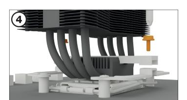
Position the cooler mounting bridge centrally on the cooler. Next place the cooler unit onto the CPU. Insert the mounting bridge fastening screws from above into the cooler mounting bridge and then screw these alternatively tight. You can use any cross-tip
